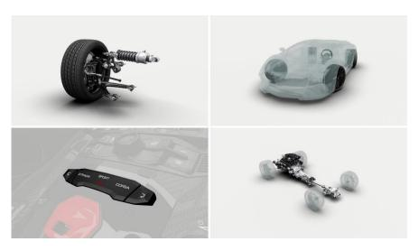
The Aventador is the first car on which Automobili Lamborghini implemented the MagneRide adaptive suspension - the first Lamborghini with rear-steering wheels.
