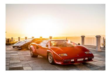
The LP 400 was replaced by the Countach LP 400 S starting from 1978. It sported the new Pirelli P7 tires, which were lowered extensively and mounted on newly designed magnesium rims,
