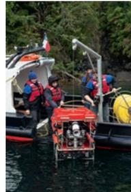
The remotely operated vehicle is placed in the water, ready for exploration.
