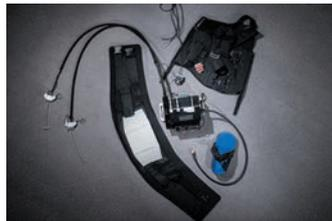
The components of an exosuit ready for assembly on a mannequin.
