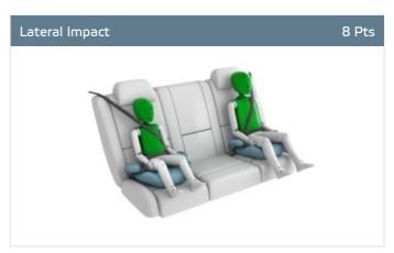
Restraint for 6 year old child: Britax Römer Kidfix i-Size (OEM) Restraint for 10 year old child: Britax Römer Kidfix i-Size (OEM) without backrest
