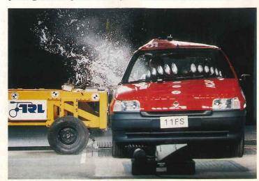
In side impact the Renault Clio failed to meet the new criteria for chest protection
