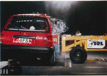
The Micra failed the new criteria for abdomen protection under side impact
