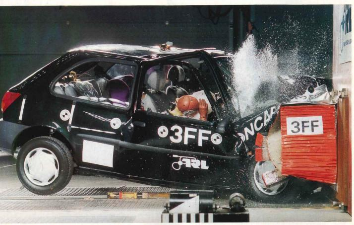
e was stable head contact on the airbag in the frontal impact crash test, during which the Ford Fiesta's passenger compartment maintained its stability
