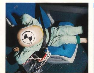
Child seat was well restrained in frontal impact but poorly in side impact. In both, the head was allowed to move too much
