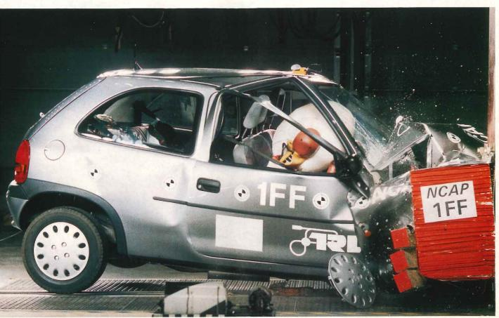
was stable head contact on the Corsa's airbag and the passenger compartment maintained its stability in frontal impact. The passenger's head hit the facia top
