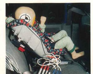
Child seat was well restrained in frontal impact but poorly in side impact. In both, the head was allowed to move too much
