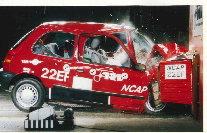
was stable head contact on the driver's airbag and the Nissan Micra's passenger compartment maintained its stability during the frontal impact crash test
