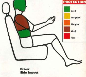
The excessive intrusion of the footwell caused the Ford Fiesta's protection of feet and ankles to be rated as weak.
