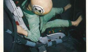
Child seat was well restrained in frontal impact but poorly in side impact. In both, the head was allowed to move too much
