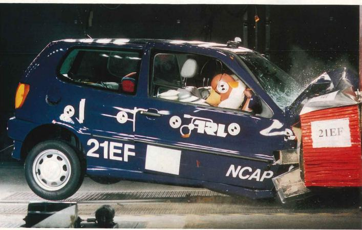
was stable head contact on the airbag in frontal impact and the VW Polo's passenger compartment maintained its stability with only limited intrusion
