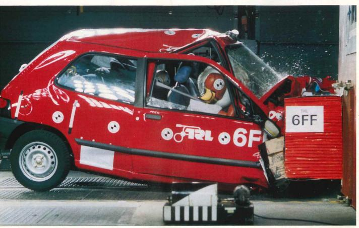
lio driver's head slid off the airbag and scuffed the windscreen pillar. The passenger compartment became unstable because of failure of welds attaching the facia
