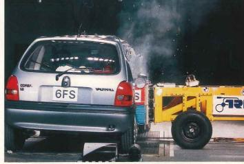
A side impact trolley with a deformable front impacts the test car at 50kph
