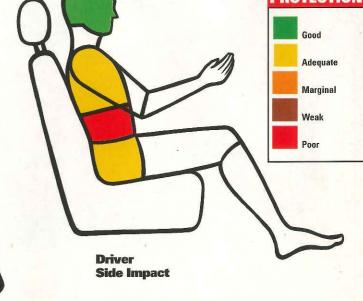
sharply increased loads. The right knee would also have received greater loading if it had impacted the facia in a slightly different position horizontally. The left knee protection was poor on the basis of dummy instrumentation and could not be downrated, but the right knee was downrated to weak to account for these points.
