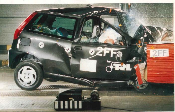
impact: head contact on the airbag was unstable and the passenger compartment became unstable due to weld failure of the A pillar and facia attachment
