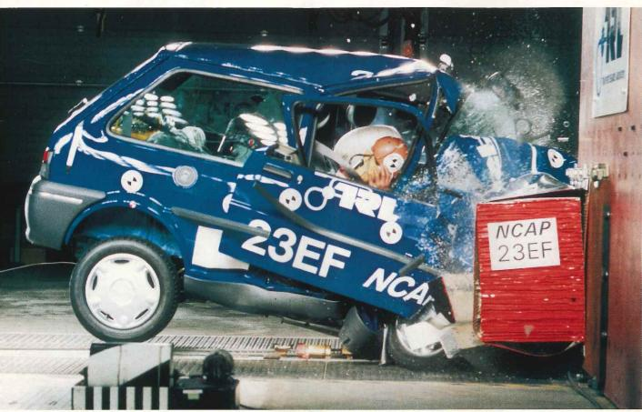
d contact with the airbag was unstable and the head struck the windscreen pillar. Passenger compartment deformation was excessive and it became unstable
