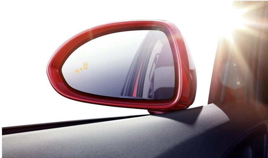
Opel Side Blind Spot Alert (SBSA) system is a technology designed to assist a driver to avoid dangerous situations or collisions with other road users during a lane change. Ultrasonic sensors scan the area to the side and diagonally to the rear of the vehicle.
