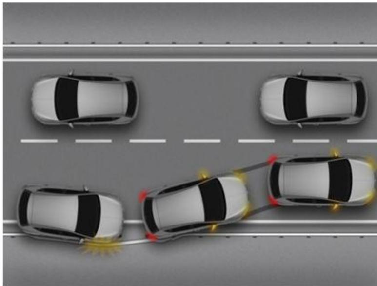
In the event of a serious primary collision, the driver will probably be unable to control the vehicle and Multi Collision Brake acts autonomously to reduce speed safely. Nevertheless, if the driver detects that braking after the initial impact is itself hazardous (for example, increasing the risk of being struck by following traffic), the system can be over-ridden by depressing the accelerator pedal.
