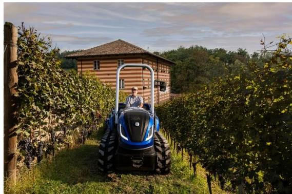
*New Holland TK Methane Power crawler vineyard tractor prototype*
