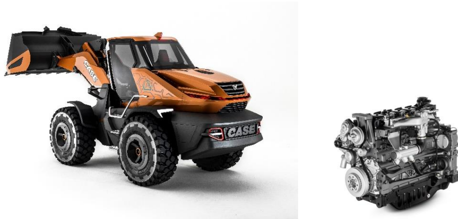
CASE Methane-Powered Wheel Loader Concept – Project TETRA and FPT Industrial 6-cylinder NG engine
