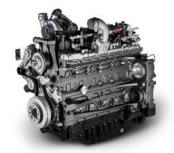
N67 NG for New Holland T6.180 Methane Power Certification: Stage V / Tier 4 Final No. of cylinders / valves: 6L / 4 Injection System: Multipoint injection Turbocharger: WG Displacement [liters]: 6.7 Bore x stroke [mm]: 104 x 132 Max power [kW] @ rpm: 130 @ 1,800 Max torque [Nm] @ rpm: 740 @ 1,500 ATS: 3-way catalytic converter
