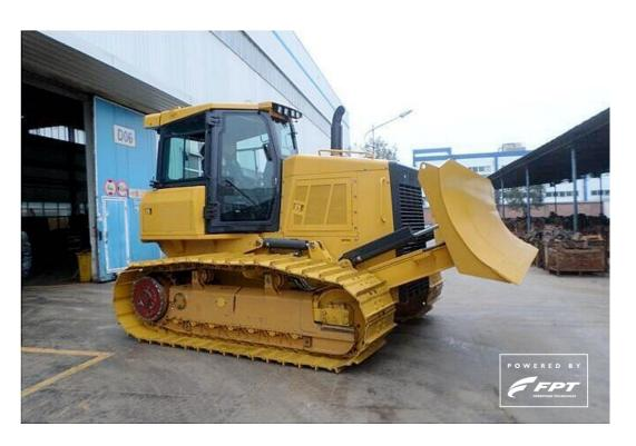
The dozers – DH13K and DH16K – are both powered by FPT Industrial NEF engines, that witnesses reliability as well as expertise and market appreciation thanks to more than 1.7 million units produced since 2011. Both these applications are equipped with N67 Tier 4 Final / Stage IV engines, which also feature the FPT Industrial patented HI-eSCR after-treatment technology. This solution is also ready for Stage V by maintaining the current cabin layout
