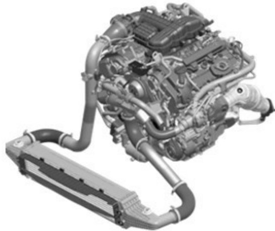
G90 3.3-liter twin-turbocharged V6 engine
