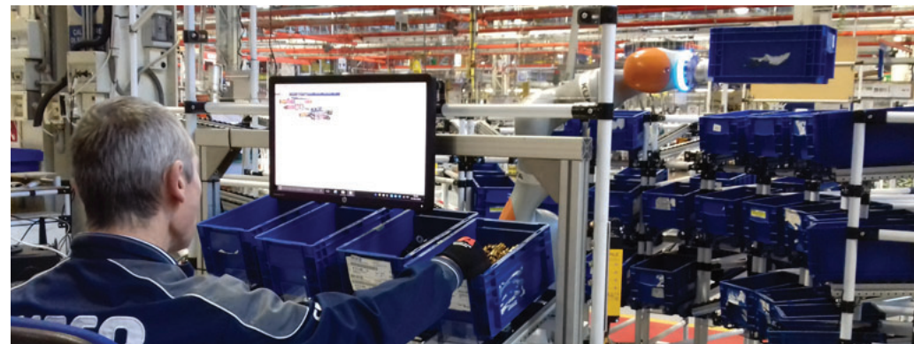
Above: the cobot collects the items and transfers them to the worker’s desk while he is comfortably seated. Left: the same job without the help of the cobot. Below left: at the Valladolid facility, automated guided vehicles move goods on the production line by the quickest route
