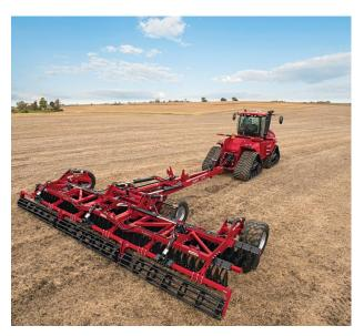
Case IH is expanding the tillage lineup with the new Speed-Tiller<sup>™</sup> high-speed disk: a true dual-season tool designed to help producers achieve productive, high-speed tillage without agronomic compromise.
