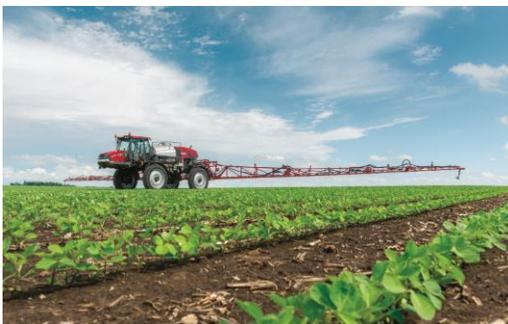
*New AutoBoom® XRT automatic boom height control, available on Patriot® and Trident™ series sprayers, is designed to increase the accuracy and coverage of applications.*
