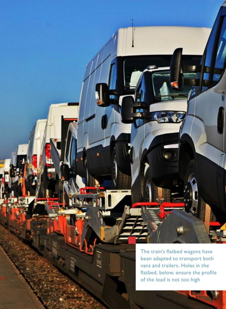
The train's flatbed wagons have been adapted to transport both vans and trailers. Holes in the flatbed, below, ensure the profile of the load is not too high
