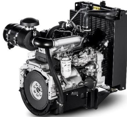
The S8000 G-Drive is developed with customers' needs in mind, providing simplicity, high power output levels and **reduced Total Cost of Ownership**. Designed for all emergency and prime power applications that do not require compliance with emission regulations, the 2.9-liter engine has a three cylinder in-line configuration for a compact architecture. This also guarantees 13% **lower fuel consumption** in comparison to competitors' four-cylinder engines.
