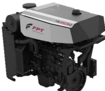
To simplify the upgrade to Stage V, FPT Industrial offers a smart installation solution, the Power Pack, which is displayed on both the F34 and the N67 engines exhibited at SIMA. In this solution, all key after-treatment components, such as DOC, SCR-on-Filter, AdBlue injection, sensors and manifolds, are fitted into one compact, pre-assembled set.
