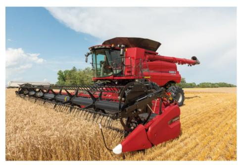
Caption: The award-winning Axial-Flow<sup>®</sup> 250 series combine features 2-speed electric shift ground drive transmission and optional AFS Harvest Command<sup>™</sup> combine automation system.
