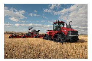
Caption: The Case IH Precision Disk™ 500DS air drill offers a one-pass solution to seed and apply fertilizer simultaneously for the highest potential crop yield.
