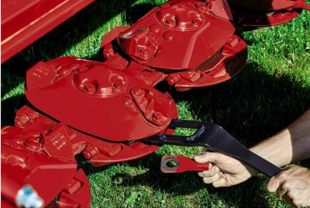
*Caption: Change knives on Case IH DC3 series disc mower conditioner headers in one-third the time of standard knife system with quick-change knives.*
