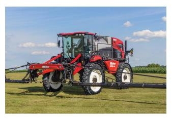
Caption: Featuring high-clearance booms with more than 6 feet of clearance and high-capacity spray tanks, the Miller Nitro® models 7370 and 7410 are engineered specifically for late-season, high-efficiency fertility and crop protection applications.
