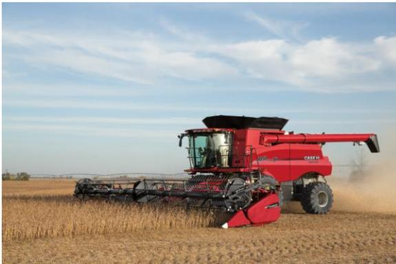
*Caption: The AFS Harvest Command™ combine automation system — available only on the new 250 series Axial-Flow® combines — proactively adjusts the combine as crop conditions change, based on patent-pending technology.*
