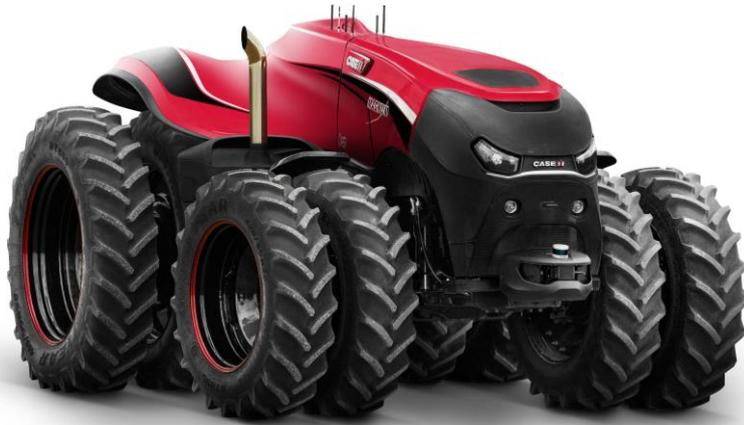
The Case IH autonomous concept tractor first debuted in August 2016 and the technology is currently being piloted on cabled tractors
