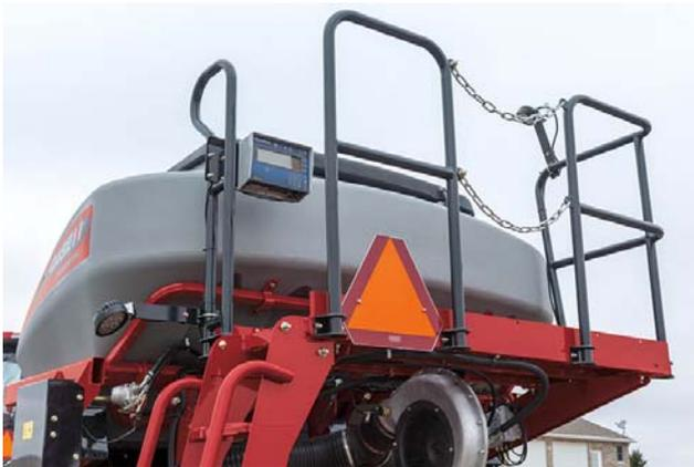
*Caption: New on the Case IH Precision Disk™ 500T single disk air drill for 2018, producers can add tank-mounted weigh scales.*
