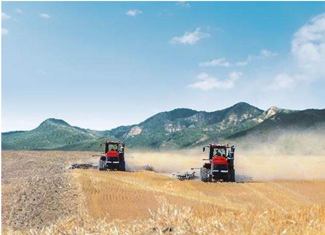
*Caption: Supervised autonomy, one of the five categories of automation as defined by Case IH, allows an operator in one tractor to supervise the operation of a tractor in the same field without an operator.*
