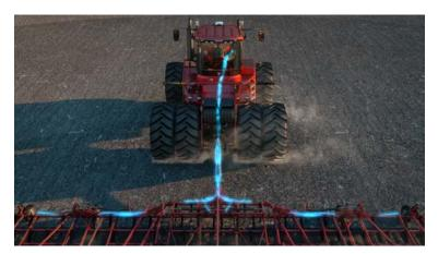
Caption: AFS Soil Command<sup>™</sup> seedbed sensors mounted on selected shank assemblies throughout the Tiger-Mate<sup>®</sup> 255 field cultivator measure the agronomic quality of the seedbed, allowing operators to adjust and optimize each tillage pass in real time.
