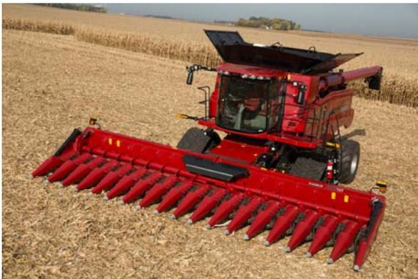
*Caption: The expanded 4400 series corn header lineup features chopping and nonchopping configurations to fit any residue management system.*
