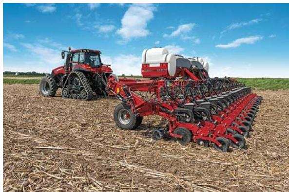
*Caption: With ultra-narrow 15-inch row spacing, the 2140 Early Riser® planter delivers two planters in one efficient machine for corn and soybean operations.*
