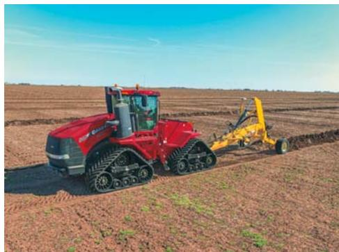
*Caption: The low-speed power of the CVXDrive™ generates increased performance and faster cycle times with reduced slippage for tile plow and scraper applications, as well as heavy-duty tillage.*
