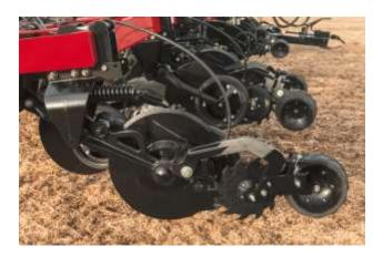
Caption: The enhanced row unit found on the Nutri-Placer 930 fertilizer applicator with new High-speed Low Disturbance (HSLD) coulter is designed to maximize productivity and crop nutrient uptake.
