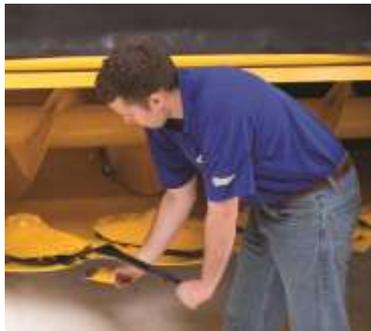
The optional **QuickMax™ quick-change knife system** provides a quick and easy method to flip or replace the cutterbar knives on New Holland Durabine® disc headers for Speedrower® self-propelled windrowers or on Discbine® 313 or 316 disc mower-conditioners. The QuickMax system greatly improves the operator's productivity because it allows a full set of cutterbar knives to be flipped or replaced in about a third of the time required to change knives on the standard, bolted, retention system.
