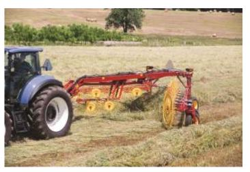
from three- to six-feet wide. The rake arms are adjustable so windrows are easily adjusted to crop and field conditions, from a fluffier windrow that promotes additional drydown to a tighter windrow to help retain moisture or reduce the potential for windrow wind damage.
