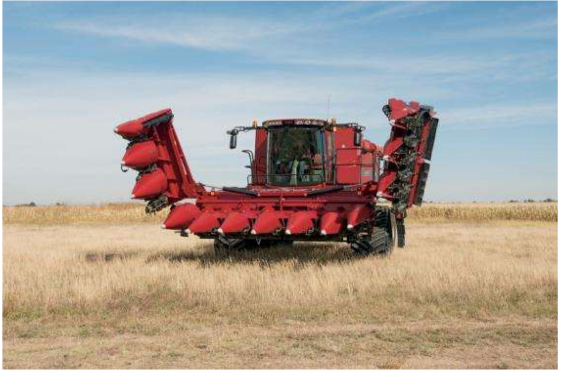
Photo Caption: The Case IH 4412F corn head is one of three Case IH products to win the prestigious AE50 award for innovative new agricultural products. The folding feature, seen in the process of folding in this photo, allows for easier transport between fields.
