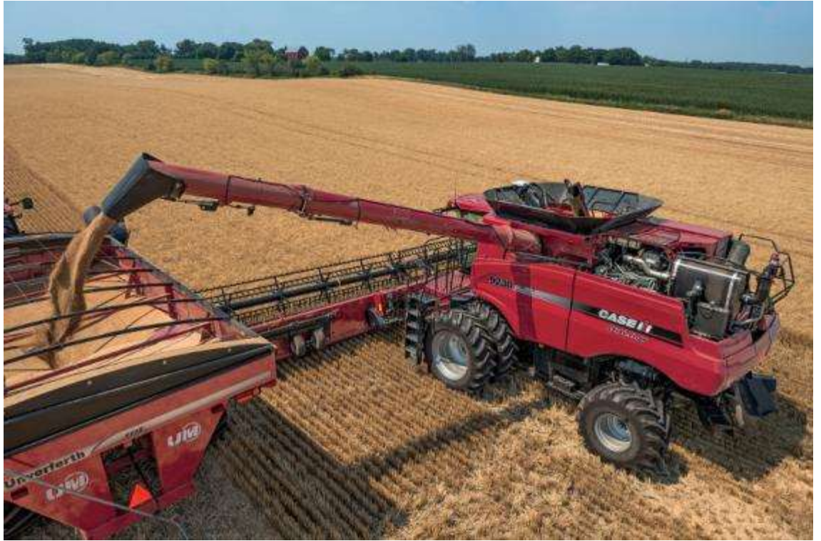
Photo Caption: Case IH Axial-Flow 230 series combines boast larger grain tanks and faster unloading speeds. The workhorses were recently recognized with an AE50 award as one of the top 50 new innovations in agriculture equipment.
