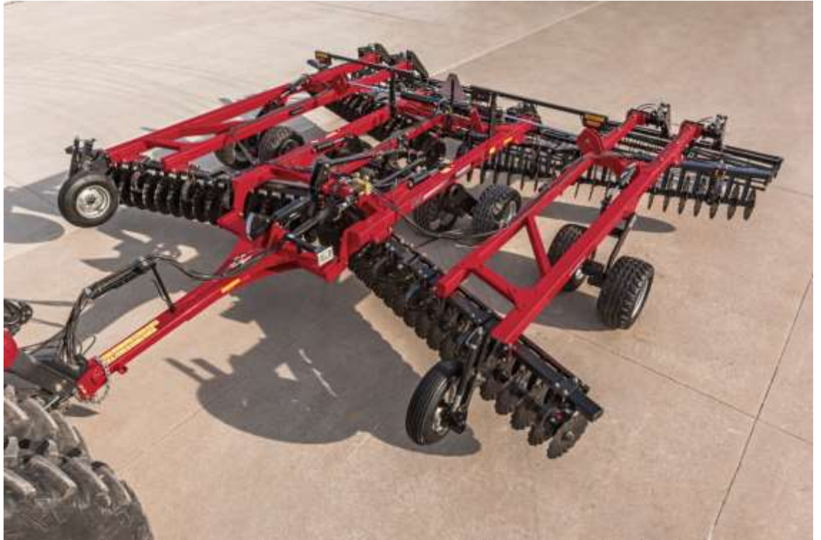
Photo Caption: Case IH introduces the new True-Tandem 335 VT vertical tillage tool, an efficient machine that covers more acres in less time, providing agronomic advantages to producers. Building on the heritage of the True-Tandem 330 Turbo, the 335 VT has an improved frame design for added durability and a hydraulic system on the rolling rear basket for control from the cab.
