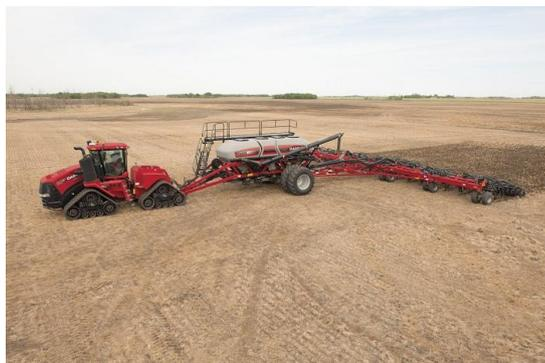
Photo caption: The new Case IH Precision Air™ 4585 air cart features a four-tank design with a total capacity of 580 bushels.
