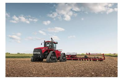
Caption: The Case IH Steiger<sup>®</sup> Quadtrac<sup>®</sup> and Rowtrac<sup>™</sup> tractors put four points of contact on the ground for increased flotation, more traction and less compaction.
