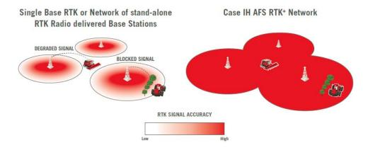
Caption: Once dealers install new Network Stations, they are networked together to provide a seamless coverage area. Case IH AFS RTK<sup>+</sup> is a cellular-based correction guidance that will provide sub-inch repeatable accuracy.
