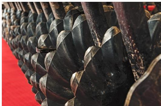
Caption: The Case IH True-Tandem™ 335 Barracuda vertical tillage system moves material up, over and laterally to stratify soil particles and increase aeration for improved soil tilth.
