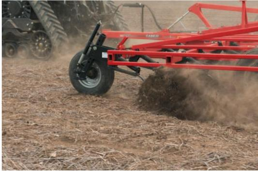
Caption: The redesigned shank assembly on the new Case IH Tiger-Mate® 255 field cultivator balances strength and flexibility to create a level seedbed at speeds up to 10 miles per hour.
