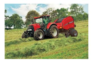
Caption: Model Year 2017 RB5 series round balers from Case IH feature ISOBUS Class 3enabled Tractor and Baler Automation technology to automatically stop the tractor when the target bale size is reached.
