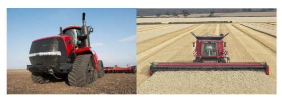
Case IH's stand at LAMMA 2014 will feature the world's most powerful tractor in series production, the 692hp Quadtrac 620, together with the world's largest combine header, the brand new 12.5m 3050 VariCut, which was developed to match Controlled Traffic Farming (CTF) systems.
