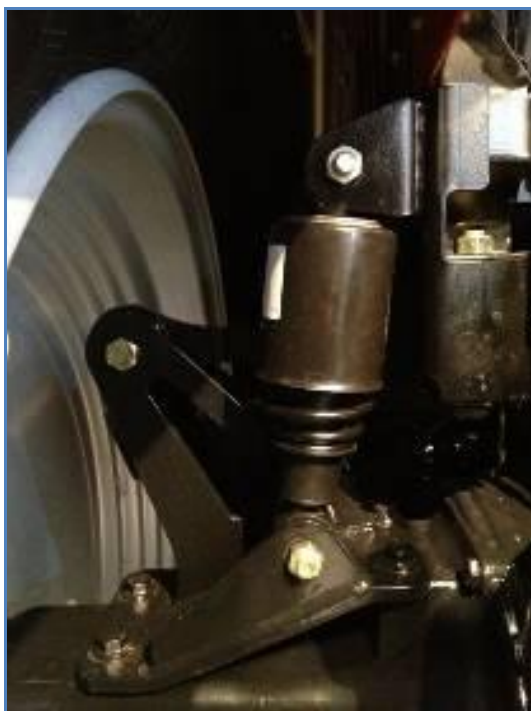
Cab suspension on Case IH Farmall U Pro
