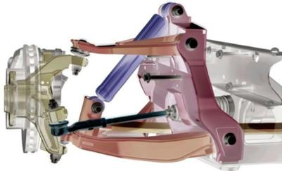
The new **QUAD LEAF front suspension** is based on a double quadrilateral arrangement with traverse leaf springs that produces excellent results in terms of containing dimensions and masses. This new front suspension, standard for all models up to 3.5 tonnes, is the best combination between the characteristics of the two previous versions thanks to several characteristics:
