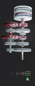
When driving, the first gear is engaged by one of the input shafts. At the same time, the other input shaft pre-selects the next gear.
