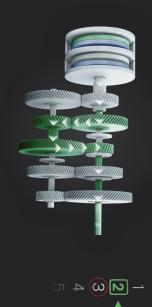
At the actual gear change, the previously engaged clutch is disengaged at the same time as the idling clutch is engaged. All without any loss of torque.
