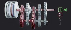
When driving, the first gear is engaged by one of the input shafts. At the same time, the other input shaft pre-selects the next gear.
