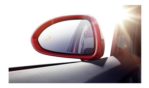
Opel Side Blind Spot Alert (SBSA) system is a technology designed to assist a driver to avoid dangerous situations or collisions with other road users during a lane change. Ultrasonic sensors scan the area to the side and diagonally to the rear of the vehicle.
