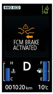
respond and the risk of collision increases, the system continues to warn the driver but also autonomously applies moderate braking, to begin to mitigate the severity of any collision but also to serve as an additional warning to the driver. If the risk of collision escalates, FCM autonomously applies a high brake pressure to try to avoid the accident or to reduce its severity. Up to 30km/h, the system will apply a maximum deceleration of 8ms-2. Beyond that speed the maximum is 6ms-2.
