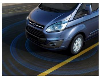
warning is given if the direction indicators are used, as the system identifies that the driver is intending to depart from the lane of travel. Similarly, if the system detects lateral accelerations above a certain level, the lane departure is assumed to be a deliberate manoeuvre by the driver.
