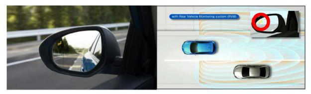
Mazda Rear Vehicle Monitoring system (RVM) is a technology designed to assist a driver to avoid dangerous situations or collisions with other road users during a lane change. Two radar sensors, one on either side of the car, are mounted in the rear bumper to measure the distance and relative speed of surrounding vehicles.
