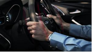
The two parts of the system can be separately turned on and off by the driver. The alert function provided by the vibrating steering wheel retains the last setting used by the driver – 'off' if the driver has previously switched it off. The steering torque is always off at the start of a journey and must be switched on by the driver if required. The system operates only at speeds above 65km/h and assists in highway driving, not in urban situations where lane crossings are frequently needed.
